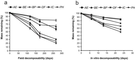
**Figure 1.** Litter mass remaining (%) as a function of decomposition time for: **(a)** field decomposability and **(b)** *in vitro* decomposability for the six herbaceous mediterranean species included in this work. n=5 for both field and *in vitro* incubation. *AE=Agrimonia eupatora, BP= Brachypodium phoenicoides, BE= Bromus erectus, DF= Dipsacus fullonum, IC= Inula conyza, PH= Picris hieracioides.*
